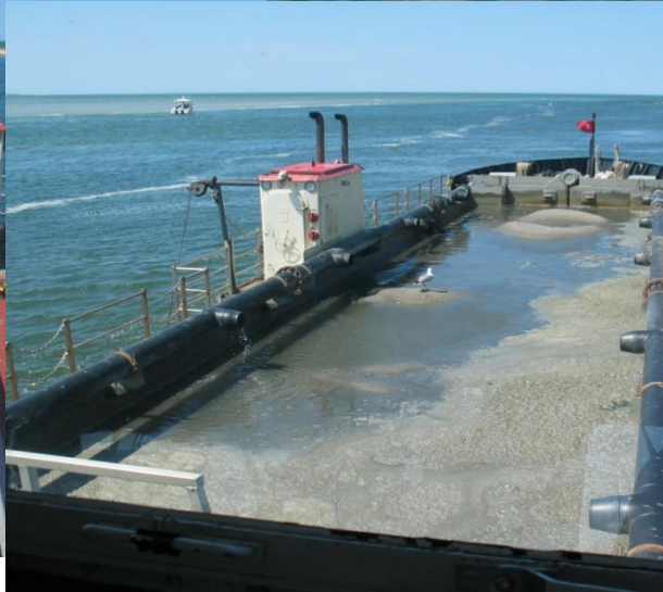
USACE Currituck Trailing Suction Hopper Dredge
