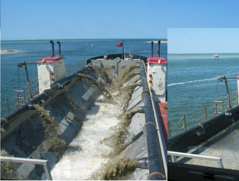
USACE Currituck Trailing Suction Hopper Dredge
