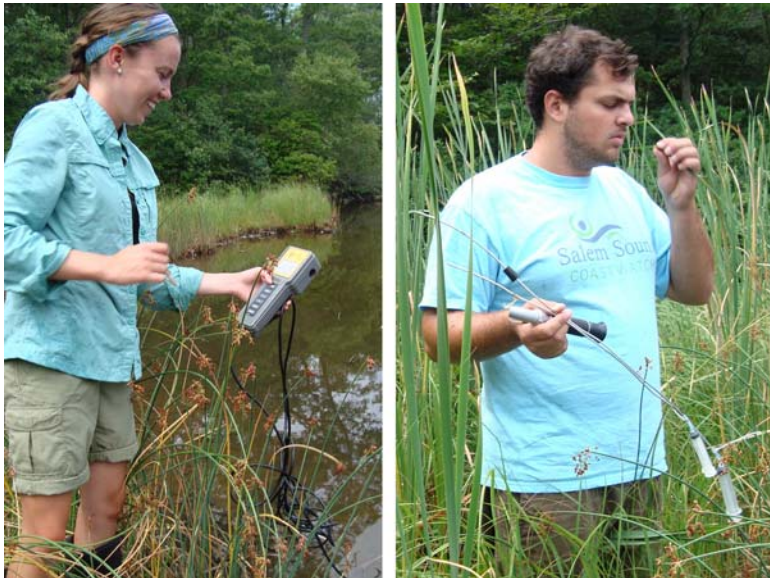
Figure 4. SSCW staff measure pond salinity with a YSI (left) and pore salinity with a sipper and refractometer (right).
